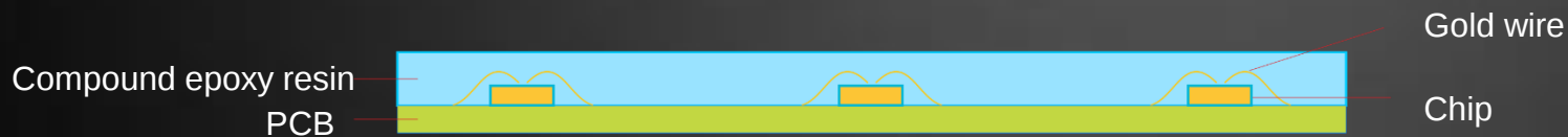
COB wire bonding process
